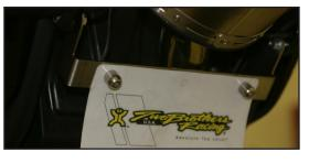
17. Attach the turn signals to their original wires. Use the supplied wire (if needed) and wire locks to attach the plate light bolts to the OEM plate light wires. Black plate lite bolt wires go to the black OEM wire and the red plate light bolt wires go to the OEM yellow wire. Zip tie together with turn signal wires and route through holes above plate.
