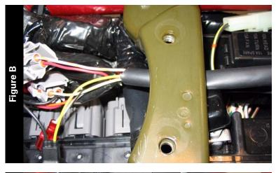
5 Route the Juice Box Pro harness under the fuel tank bracket as shown in Figure B.
