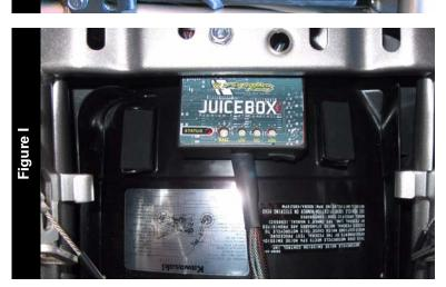
19 Using the stock rubber band, secure the Juice Box Pro in the tail section.
