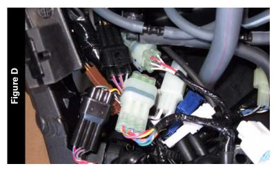
Attach the connectors from the Juice Box Pro to the stock wiring harness and the throttle bodies as shown in Figure D.
