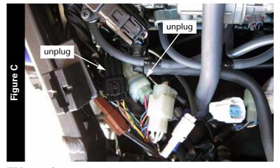
Unplug the two 6-pin connectors from the throttle bodies as shown in Figure C.
