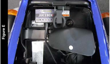
10 Using the supplied velcro, secure the Juice Box Pro in the tail section as shown in Figure E.
