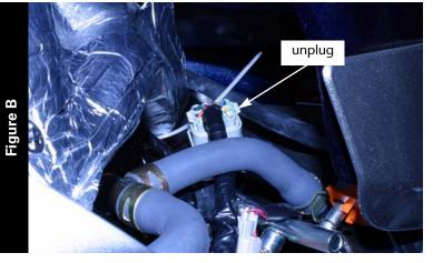
7 Unplug the stock connector from the throttle bodies to the main wiring harness as shown in Figure B.
