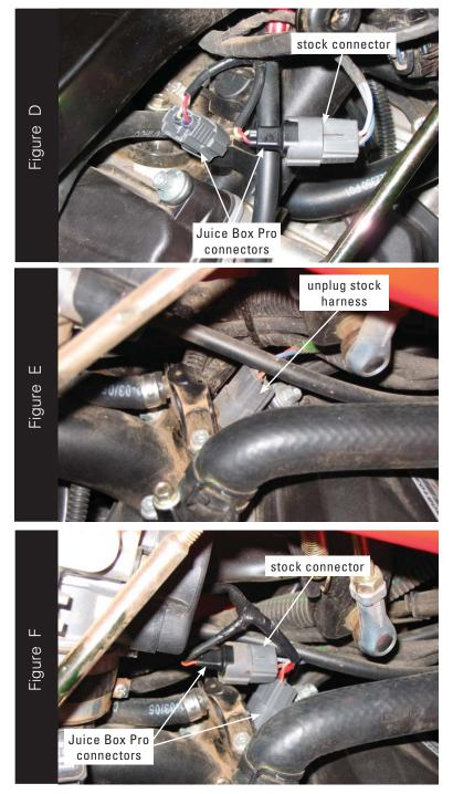
6. Attach the yellow colored wires from the Juice Box Pro to the stock wiring harness and the rear fuel injector as shown in Figure D.
