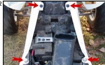
5. Remove the 2 fuel tank mounting bolts and 2 plastic screws that are holding the rubber flap (Figure 3).
