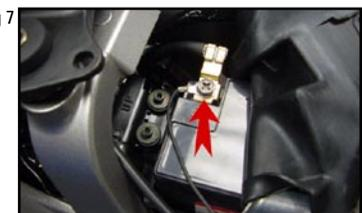
11. For tuning purposes you may want to keep the JUICE BOX™ where you can reach it. Once you get things dialed in, route the JUICE BOX™ wire harness under the battery mount and the two air box mounting tabs then secure the harness to the frame with zip ties. The JUICE BOX™ will easily fit in the rear toolbox area with the supplied Velcro pad. (Figure 8)
