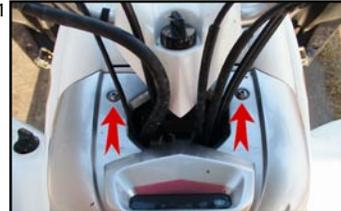
4. Remove the 2 bolts holding the side panels and 2 plastic screws (Figure 2).
