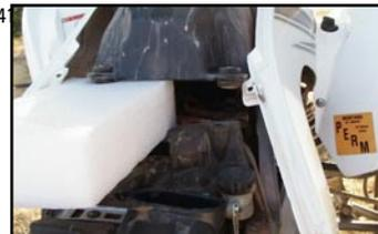
7. Remove the stock fuel injector connector at the fuel injector (Figure 5).
