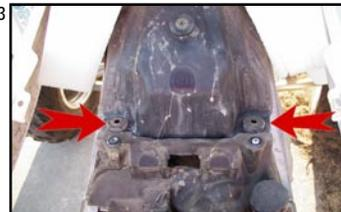
6. Lift the tank up; you do not need to remove it (Figure 4) and support with foam block from TBR exhaust packaging.
