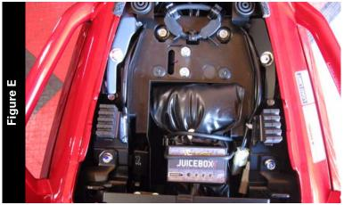
11 Using the supplied velcro, Install the Juice Box Pro in the rear section of the trunk as shown in Figure E.
