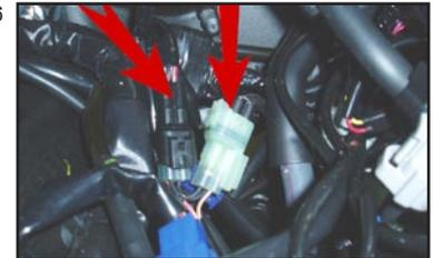
8. Tuck the wiring in to prevent pinching under the tank. (Fig 7)
