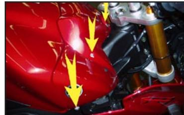
4. Remove the 2 front fuel tank fasteners. (Fig 3)
