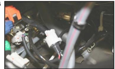
7. Disconnect the Oxygen sensor connector and install the JUICE BOX™ harness. (Fig 6)
