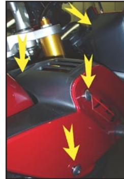
3. Remove the 5 fasteners and remove the tank apron. (Fig 2)
