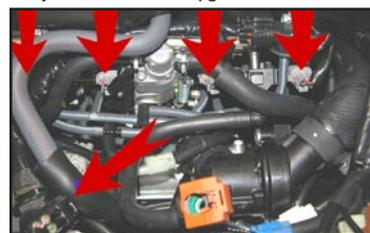
6. Remove the injector connectors one at a time. Connect the JUICE BOX™ harness to the injector, and the stock injector connector to the JUICE BOX™ harness. (Fig 5)
