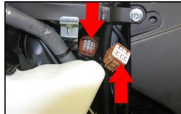
5. Connect the JUICE BOX™ connectors to these connectors. Route the JUICE BOX™ harness along the main stock harness and up to the front of the bike. Attach the ground lead (black wire) to the silver bracket with bolt that attaches to the frame near where the ram air tube enters the air box. (Fig 4)
