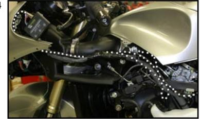
6. Attach the adhesive backed hook and loop material to the back of the JUICE BOX™ and the black left side trim panel just left of the instrument cluster. (Fig 5)
