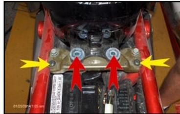
4. Lift gas tank up gently just enough to access to the quick disconnect and release the red lock tab and remove fuel line (Fig 2). Remove any and all vent lines from the tank. Gently remove gas tank and set aside.
