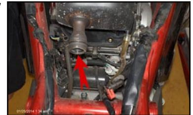
7. The JUICE BOX™ will be placed under the seat so you need to thread the JUICE BOX™ wires towards the front of the bike under the gas tank support plate towards the throttle bodies. You can remove the tank support plate by removing the 2 10mm bolts (Fig 8). Locate the injector connectors and disconnect the stock connectors and plug the JUICE BOX™ grey connector onto the bikes injector, and then plug the stock connector into the JUICE BOX™ black connector repeat on remaining cylinder (Fig 9).
