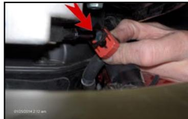
5. Disconnect fresh air system hose from the fresh air solenoid then disconnect the black air temp connector (Fig 3). Disconnect the green connector from the solenoid then remove solenoid from air box (Fig 4). Remove all of the air box screws 7 total (Fig 5) and remove lid.
