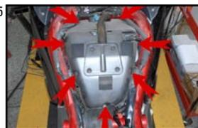
6. Remove the 4, 5mm Allen bolts, (Fig 6) and while lifting air box lid you will need to disconnect the crankcase breather hose from the gearbox (Fig 7).
