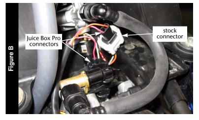
Attach the connectors from the Juice Box Pro to the stock wiring harness and the fuel injector as shown in Figure B.
