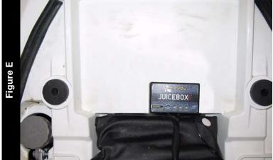
11 Using the supplied velcro, secure the Juice Box Pro to the rear fender as shown in Figure E.
