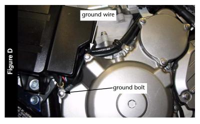
10 Attach the ground wire from the Juice Box Pro to the common ground on the left hand side of the engine as shown in Figure D.
