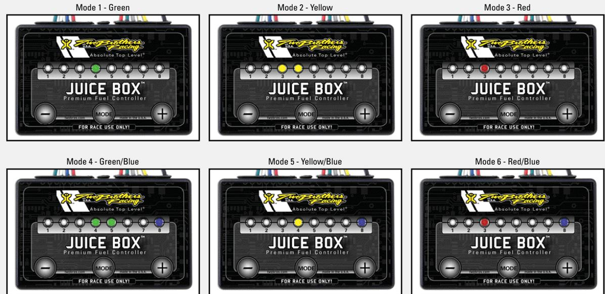
**GSX-R750 Pre-set Settings:** GSX-R750 baseline settings with stock air filter and TBR slip-on system. (G=2.5, Y=3.5, R=3, GB=2, YB=4, RB=3)
