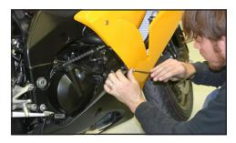
Remove right side rear pasenger peg, heat shield and heat shield cover. 7. Remove right side peg assembly.
