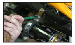
21. Making sure that muffler orientation is correct, tighten upper muffler mount bolt, then tighten the 4 6x14mm V.A.L.E. bolts. Then tighten lower muffler mount on lower S-bend.
