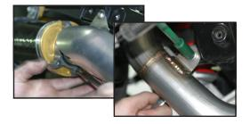
22. Tighten the 2 barrel clamps joining the pipes together.
