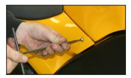
Remove rear cowling by removing bolts and push pins that attach to frame.
