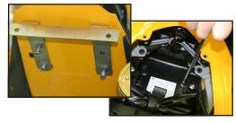
26. Use supplied Lite'n-bolts to attach license plate to license plate bracket and connect wires using supplied scotch locks to the red and black license plate wires on left side of rear cowling area. Use included adhesive tab and zip tie to keep wires contained. Check that plate lights light license plate with key on.
