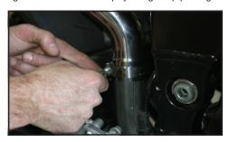
Reinstall swingarm pipe cover, foot peg assembly, and heat shield. 24. Reinstall heat shield cover and passenger peg assembly.
