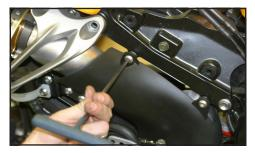
25. Install supplied license plate bracket onto rear tail section using the 4 6x16mm socket head cap screws and washers.
