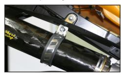
19. Slide lined muffler clamp over muffler and install muffler assembly onto S-bend-1 using your second barrel clamp between upper and lower S-bend.
