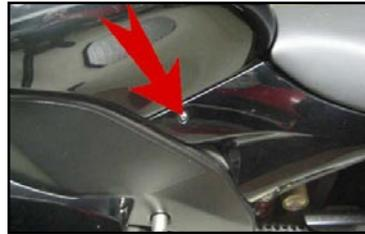
3. Remove seat mount screws, remove seat. (Fig 2)
