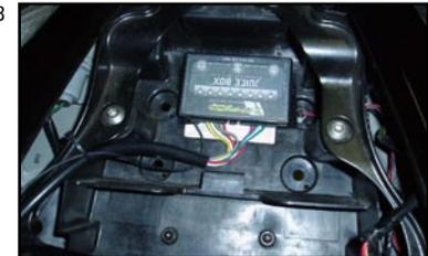
NOTE: Re check your wire routing and JUICE BOX™ location and make certain that in no way the wires can come into contact with any moving parts or high heat source and that the JUICE BOX™ is mounted in a way as to not cause a handling problem with the machine.
