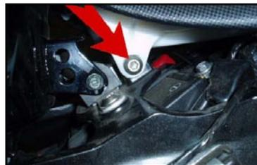
4. Remove front tank stay bolts. Lift and support tank. (Fig 3)
