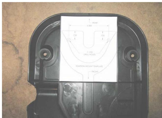
6) Use template to drill the two ignition mounting holes
