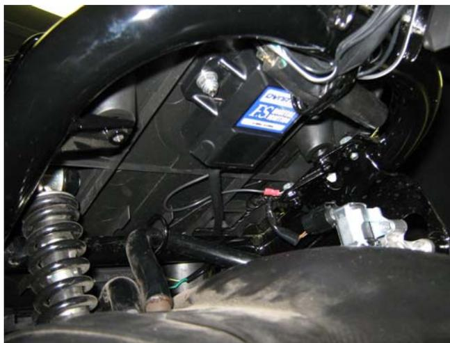
**Final Ignition Mounting is under the rear deck.**
