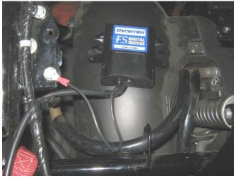
1) Ground Connection – note: not final ignition mounting 2) Pickup connection
