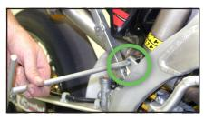
9. Securely tighten the 4 (four) 6x14mm hex head bolts of the V.A.L.E. assembly.
