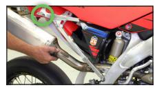
Use the 4 (four) 6x14mm socket head cap screws and lock washers to loosely attach the X-Lite<sup>™</sup> ring to muffler inlet.
