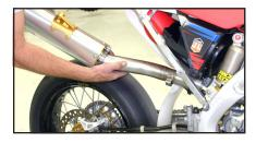
7. Attach muffler mounting bracket to mounting tab on subframe using supplied 8x25mm bolt. Leave loose for now.
