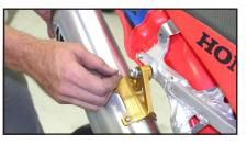
8. Using OEM bolt, secure muffler assembly mid-pipe bolt. Tighten securely.
