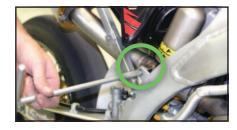
4. Remove upper muffler mounting bolt and muffler assembly.
