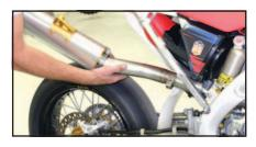
8. Attach muffler mounting bracket to mounting tab on subframe using supplied 8x25mm bolt. Leave loose for now.
