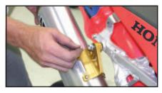
9. Using OEM bolt, secure muffler assembly mid-pipe bolt. Tighten securely.
