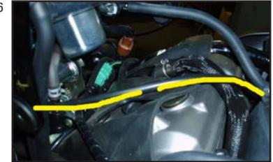
8. Locate the throttle body harness connector, it's between the LH frame and airbox. Reach in through the LH frame opening, find and disconnect. Pull the JUICE BOX™ harness connector out through the frame opening.
