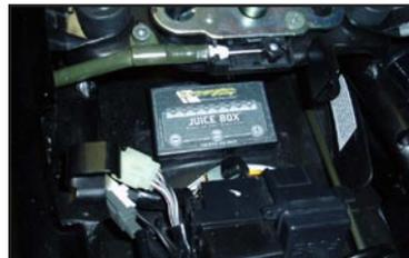
6. Route the harness down the RH frame. connect ground to the negative post of the battery. (Fig 5)
