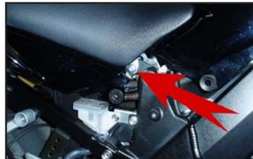
4. Remove front tank mount hardware, lift and support tank. (Fig 3)
