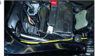
7. Route harness over rear cylinder head and down the left side of the throttle body. (Fig 6)
