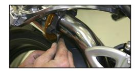
Tighten the muffler clamp, securely attaching the muffler assembly to the bike.
