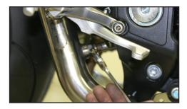
11. Make sure position of muffler is correct. Once you are satisfied with its position, tighten X-Lite™ ring bolts on the V.A.L.E.™ assembly.
