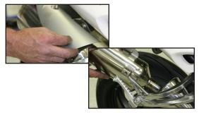
3. Loosen stock  $O^2$  sensor and barrel clamp and remove the rear s-bend section.
