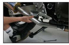
Slip the supplied rubber lined muffler clamp onto the muffler canister and loosely attach to the upper mount behind the rear passenger peg using the stock hardware. 6. With the new exhaust assembly in place, securely tighten the 4 V.A.L.E. socket head cap screws, securing the X-Lite retaining ring and exhaust tube to the muffler canister, keeping sure that the muffler is in correct alignment with the bike.
