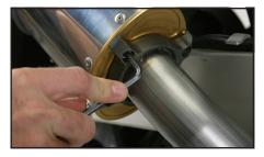
7. Securely tighten the muffler canister clamp.
