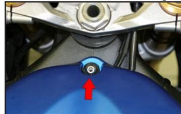
5. Gently raise fuel tank up and support it with a suitable object then disconnect fuel line, fuel pump wire and vent hoses. Remove fuel tank.
