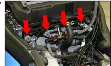
8. Disconnect injector connector and plug the grey JUICE BOX™ connector onto the injector and pig tail black connector into the OEM grey connector (Fig 8). Repeat on remaining 3 cylinders.
