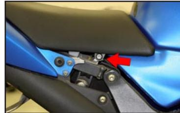
4. Remove tank bolt from front of fuel tank. (Fig 4)
