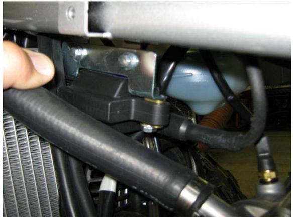
Step 4: Mount coil bracket to frame.
