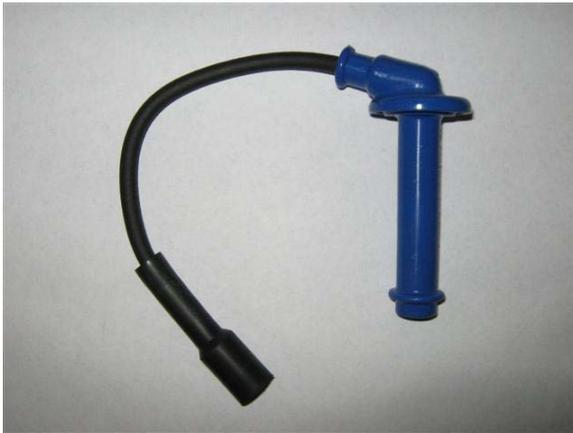
Step 1: Spark plug wire assembled.
