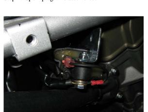
Step 3: Attach ground wire to Red dot terminal. Black/yellow wire to terminal without mark.
