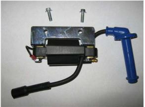
Step 2: Assemble Dyna coil, bracket, and hardware.
