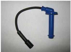
Step 1: Spark plug wire assembled.
