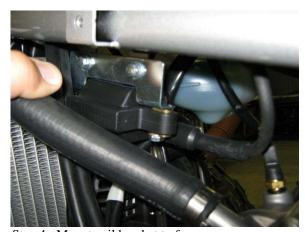
Step 4: Mount coil bracket to frame. Attach wire to coil and sparkplug.
