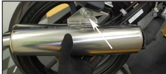
3. Install the canister onto the end of the stock exhaust flange (the TBR badge faces to the outside). You'll have to hold it in place while you start the OEM bolts through the flange holes and into the inlet. Go ahead and tighten evenly and fully. (Use Hi-temp silicone on gasket.)
