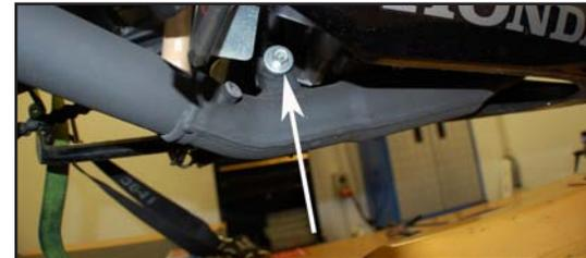
6. Before you run the bike, clean off all fingerprints and dirt, as any oily residue will etch the metal and become somewhat permanent when the system gets hot. Run the bike and enjoy. It is normal for some white smoke to appear the first time you start the bike. This is packing/manufacturing oil from inside the pipe burning off. Check for gaps or leaks. If you find a leak, a little high temperature silicon sealant should fix it. After 50 to 100 miles, recheck all fasteners for tightness.
