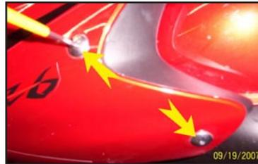
4. And remove fairing section (Fig 2). Perform on right hand side also.
