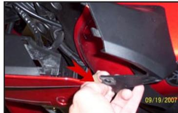
5. Remove the two front gas tank mounting bolts (Fig 3). Gently raise the gas tank up and support with suitable prop rod.
