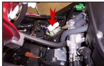
7. Route the Juice Box harness from the left side, rear of the tank toward the white sub harness connector along the bikes stock wiring loom, secure with ties.
