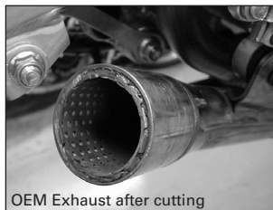
OEM Exhaust after cutting
