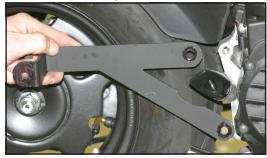
Install TBR Header pipe using the OEM gasket between header pipe and cylinder head, use OEM bolts.
