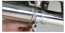
Slide muffler clamp over muffler and attach to muffler mount using OEM hardware. Muffler clamp tabs should be to the back of the mount.
