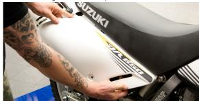
Remove plate to access joint clamp.
