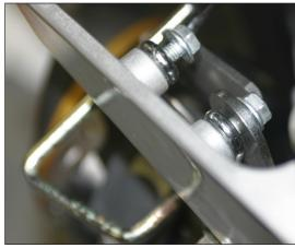
Loosely attach the V.A.L.E.™ muffler to the stainless steel V.A.L.E.™ connector tube using the supplied 6x20mm socket head cap screws and 6mm split washers.
