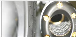
11. Tighten X-ring bolts then barrel clamp.
