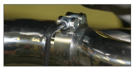
12. Before you run the bike, clean off all fingerprints and dirt, as any oily residue will etch the metal and become somewhat permanent when the system gets hot. Run the bike and enjoy. It is normal for some white smoke to appear the first time you start the bike. This is packing/manufacturing oil from inside the pipe burnin g off. Check for gaps or leaks. If you find a leak, a little high temperature silicon sealant should fix it. After 50 to 100 miles, recheck all fasteners for tightness.
