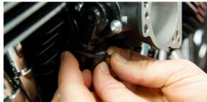
3. Disassemble Comp-V to backing plate.
