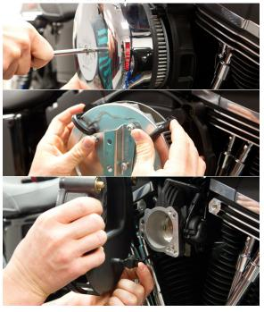
2. Remove plug from back of OEM backing plate and zip-tie out of way.
