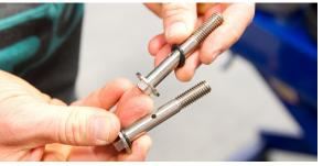
5. Install one o-ring onto each end of the oil-channel spacer.
