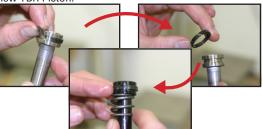
Install your new piston by pushing it in using the spring.
