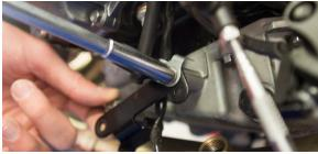
Loosely install the TBR slip tube and barrel clamp to the TBR headers.
