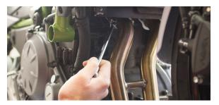
Remove O2 sensor routing bracket. Re-install side covers and check for clearance. When muffler is positioned tighten barrel clamp at header joint.
