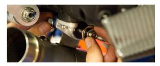
Attached supplied TBR Muffler mounting bracket using the OEM bolt and supplied 8mm nut to OEM Mounting points behind the rearset.
