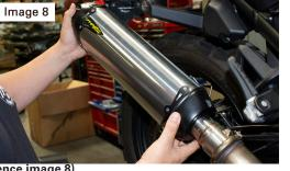
. Install muffler onto pre-installed slip-tube. (Reference image 8)
