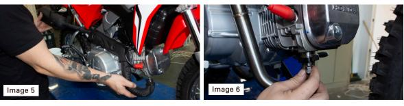
Install muffler to the OEM mounting point and TBR header pipe using OEM muffler bolt. (Reference image 7 & 8) 8.
