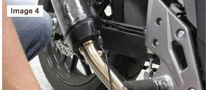
5. Using the supplied hardware install the muffler clamp as shown. Use the included spacer between the clamp and passenger peg bracket. (Reference image 5)
