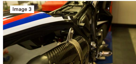
5. Install the supplied springs, attaching the muffler to the slip tube.
