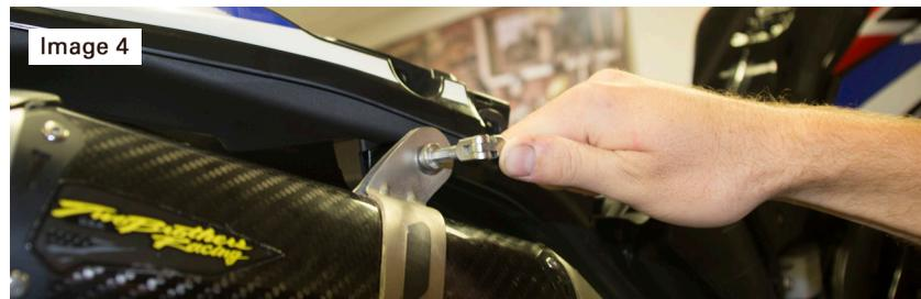
7. Before you run the bike, clean off all fingerprints and dirt, as any oily residue will etch the metal and become somewhat permanent when the system gets hot. Run the bike and enjoy. It is normal for some white smoke to
