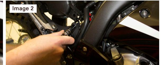
3. Remove upper muffler bracket bolt located just below the seat on the Rally or behind the number plate for the standard CRF250L model.
