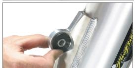
4. Attach slip tube to TBR muffler using the supplied springs.
