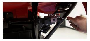
Assemble the TBR exhaust pieces using the supplied springs as shown in the picture.
