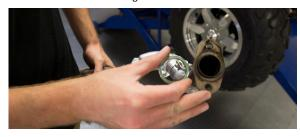
Using the OEM bolts, loosely install the supplied TBR brackets, replacing the OEM exhaust brackets as shown.
