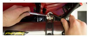
Install the supplied springs to attach the muffler to the exhaust.
