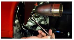
14. Install the S1R Canister onto the exhaust.
