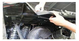
7. Install the TBR bracket under the panel support bracket and secure it using the 2 black nuts.
