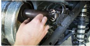
3. Remove the OEM exhaust mounting bracket bolts and rubber mount isolator.
