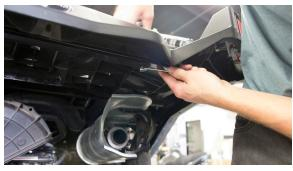
8. Attach the slip tube to the existing exhaust using the supplied Barrel Clamp.
