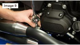
9. Before you run the bike, clean off all fingerprints and dirt, as any oily residue will etch the metal and become somewhat permanent when the system gets hot. Run the bike and enjoy. It is normal for some white smoke to appear the first time you start the bike. This is packing/manufacturing oil from inside the pipe burning off. Check for gaps or leaks. If you find a leak, a little high temperature silicon sealant should fix it. After 50 to 100 miles, recheck all fasteners for tightness.
