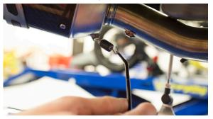
13. Reinstall O2 sensor onto TBR slip tube using supplied 12mm adapter kit and copper washer.
