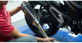
Attach TBR muffler system to motorcycle using OEM hardware on lower mount with supplied 10mm nut. Use 8x75mm socket head cap screw and 18mm spacer with 8mm nut on muffler mount.
