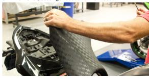
Remove body work from right side of motorcycle to accesss butterfly valve servo cables.
