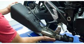
Attach TBR slip tube to TBR muffler using the supplied springs.
