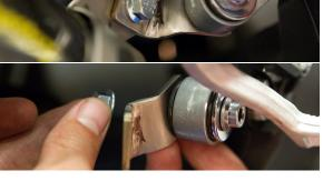
18. Attach TBR slip muffler assembly to y-pipe using supplied springs.
