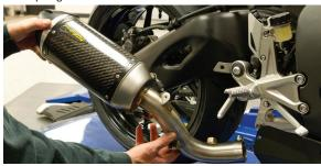
Slide rubber-lined muffler clamp over TBR exhaust canister, loosely slide the barrel clamp over the slip-tube. Install the muffler assembly to the bike by attaching the muffler clamp to the custom bracket using the supplied counter-sunk washer, bolt and nut.
