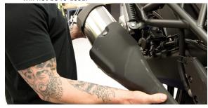
Install Two Brothers Racing Slip-on Exhaust System: Attach the mid-pipe to the muffler using the 2 hook springs provided. Apply a thin layer of anti-seize to muffler inlet.
