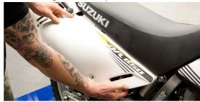
Remove plate to access joint clamp.
