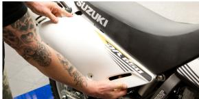
3. Remove plate to access joint clamp.
